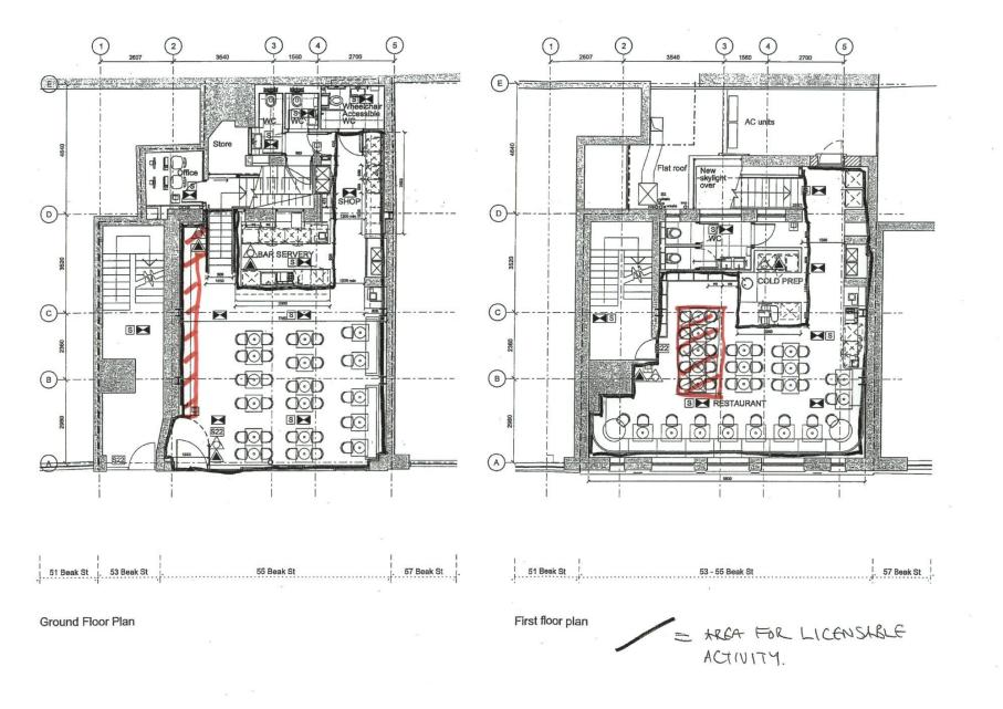
FIRE SAFETY LEGEND Fire alarm call point Fire alarm bell sounder Fire extiguisher Carbon Dioxide Fire Exit sign with emergency light Fire Exit sign with arrow indicating direction of escape route **DESIGN INTENT ONLY** mackay partners 63 Gee St, London EC1V 3RS tol +44 (0)207 508 1177 Vinoteca Beak Street Proposed Plans Ground and First Floor with Fire Strategy
